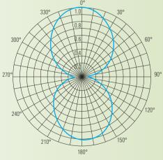
Typical radiation pattern in the E plane at 500 MHz
