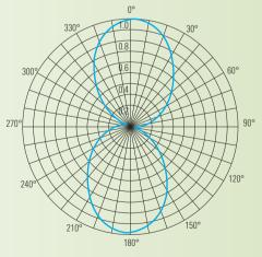
Typical radiation pattern in the E plane at 200 MHz
