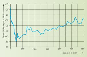
Typical field-strength sensitivity at antenna output (measurement bandwidth  $\Delta f = 1$  Hz; S/N = 0 dB)
