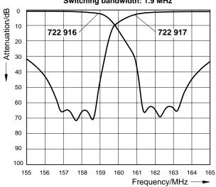
Band spacing: 6.0 MHz Switching bandwidth: 1.0 MHz
