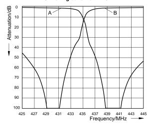
Duplex spacing : 10 MHz Switching bandwidth: 4.0 MHz
