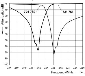
Band spacing: 10 MHz Switching bandwidth: 1.0 MHz
