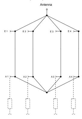
Connectors E 1 ... E 4: Inputs, decoupled Connectors A 1 ... A 4: External  $50-\Omega$  absorbers
