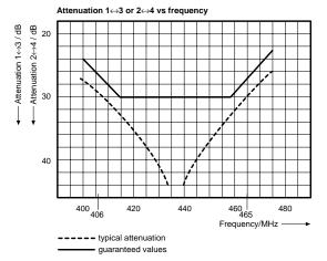
The remaining ports are terminated with  $50-\Omega$  loads.
