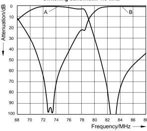
Duplex spacing: 9.8 MHz Switching bandwidth: 2.5 MHz
