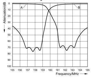
Duplex spacing: 6.0 MHz Switching bandwidth: 1.0 MHz
