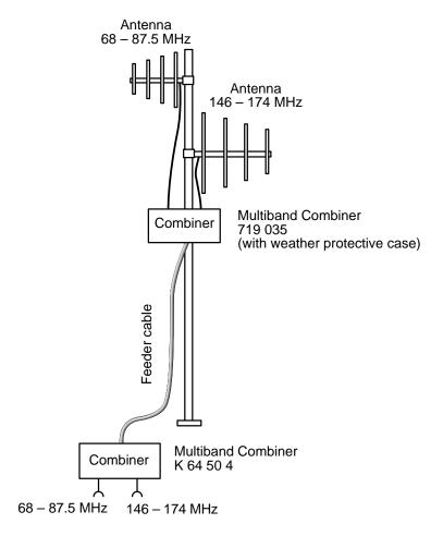
Example for the combining of 80 MHz and 160 MHz tansmitters/receivers to a common feeder cable
