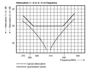
The remaining ports are terminated with  $50-\Omega$  loads.
