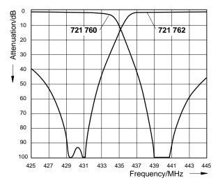
Band spacing: 10 MHz Switching bandwidth: 4.0 MHz
