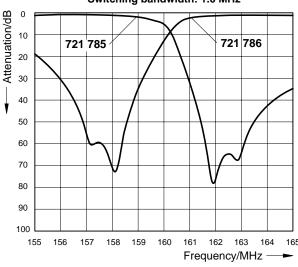
Band spacing: 4.6 MHz Switching bandwidth: 1.9 MHz
