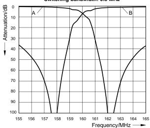
Duplex spacing: 4.6 MHz Switching bandwidth: 1.0 MHz
