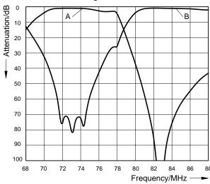
Duplex spacing: 9.8 MHz Switching bandwidth: 4.0 MHz
