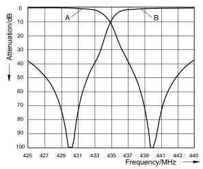
Duplex spacing: 10 MHz Switching bandwidth: 2.0 MHz
