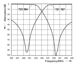
Band spacing: 10 MHz Switching bandwidth: 2.0 MHz
