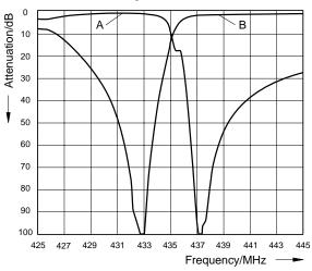
Duplex spacing : 10 MHz Switching bandwidth: 2.0 MHz
