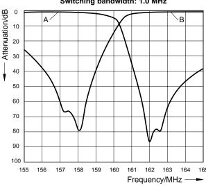
Duplex spacing: 4.6 MHz Switching bandwidth: 1.9 MHz
