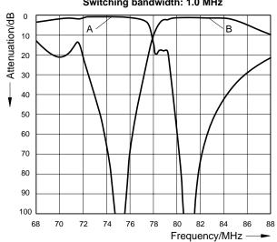
Duplex spacing: 9.8 MHz Switching bandwidth: 1.0 MHz
