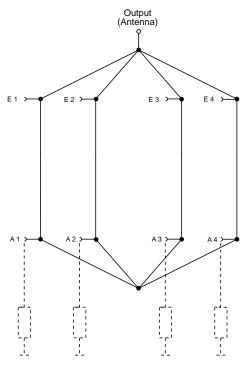
Connectors E 1 ... E 4: Inputs, decoupled Connectors A 1 ... A 4: External  $50-\Omega$  absorbers
