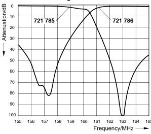
Band spacing: 6.0 MHz Switching bandwidth: 2.0 MHz
